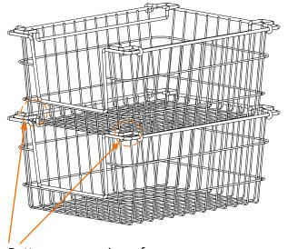
Note: Bottom corner wires of top basket interlock onto handle wires of lower basket.
