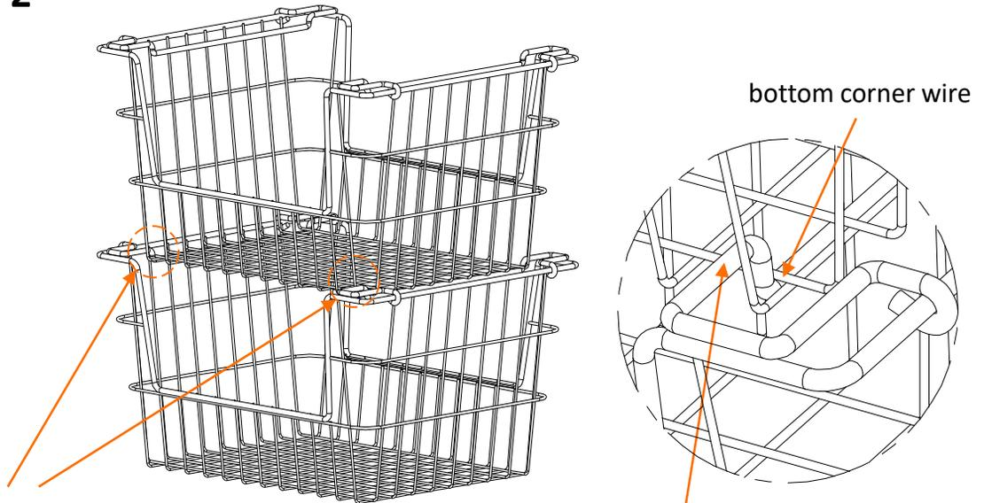
Note: Bottom corner wires of top basket interlock onto handle wires of lower basket.
