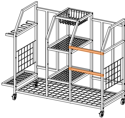
Option 2 : Front bar on one side, 1 middle position ,1 higher position for tall items.
