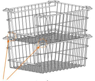
Note: Bottom corner wires of top basket interlock onto handle wires of lower basket.
