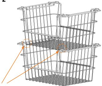
Note: Bottom corner wires of top basket interlock onto handle wires of lower basket. bottom corner wire
