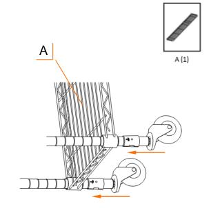
\*\*\*For convenience, place BOTTOM POLES (F) with Locking Casters on the long side of the shelf if the organizer will be pushed against a wall OR if the organizer is frequently rolled around like a cart, place BOTTOM POLES (F) with Locking Casters on the side being pushed or pulled.
