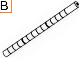
BACK BOTTOM POLE (2) Threaded Insert (2), Pole Connector (2) and Feet Leveler (2) are pre-installed
